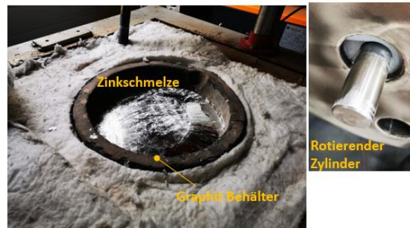
Figure 2: Photo of the RDE test set-up with the molten zinc and the rotating cylinder. Picture: MUL-NEM
