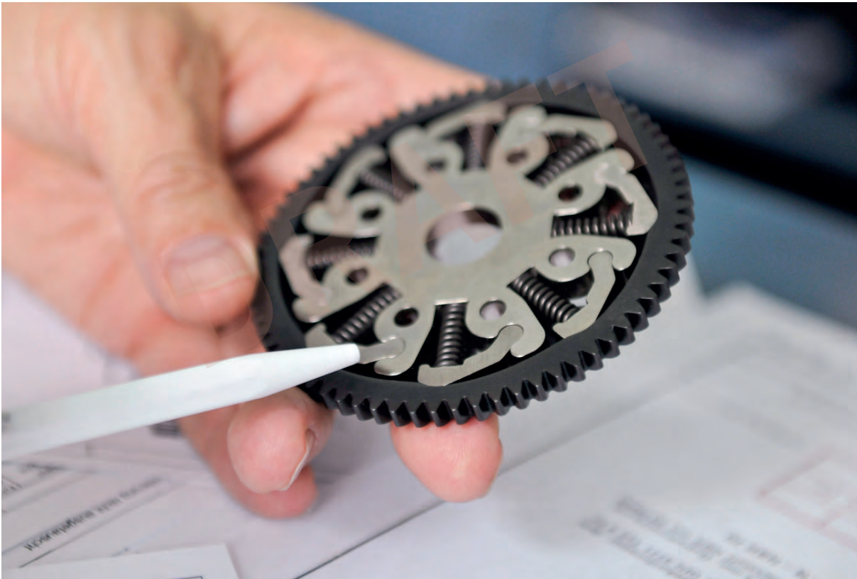
Fig. 1: Parts that are produced via fine blanking today (© Fritz Schiess AG, CH-9620 Lichtensteig)
