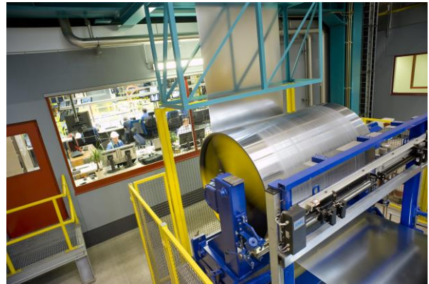
View of the control station of the hot-dip galvanizing line. In the foreground you can see the steel belt with deflection roller. © voestalpine
