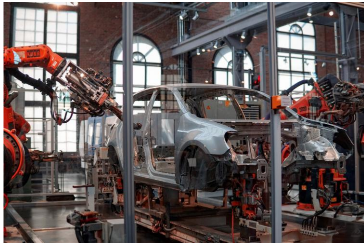
Image 1: Car body spot welded by robots. © Photo by Lenny Kuhne on Unsplash
