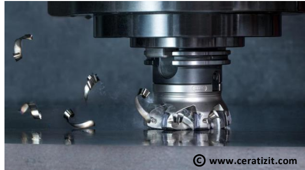
Milling tool equipped with indexable inserts during application
