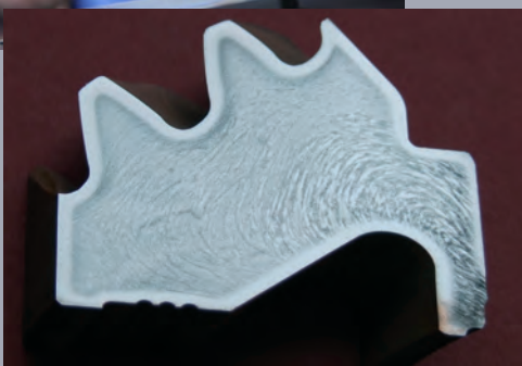
Macroetching of cross-section of a toothed wheel
