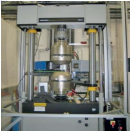
Specially adapted facility for standardised testing of materials at stresses of approx. 10,000 MPa
