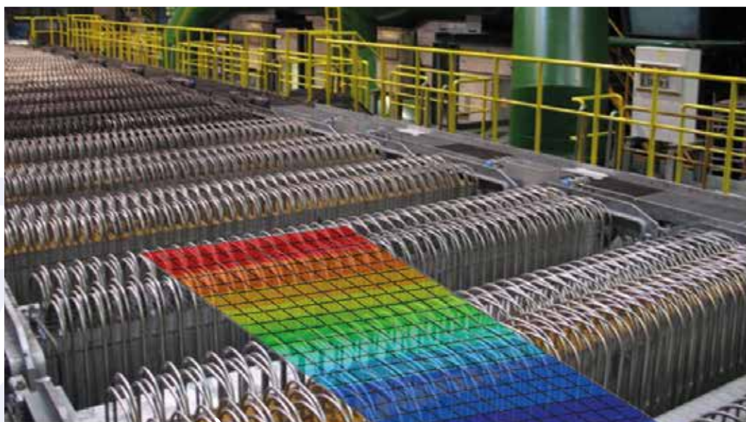
Accelerated cooling line of voestalpine Grobblech GmbH and superimposed 3D finite element model with the colour coding denoting the temperature field
