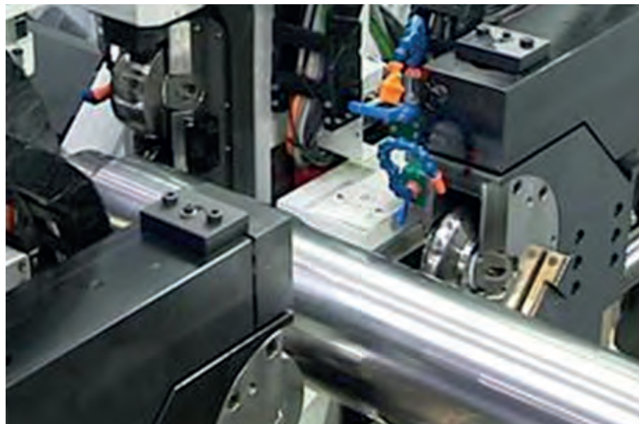
Deep rolling a wheelset axle (Source: Hegenscheidt)
