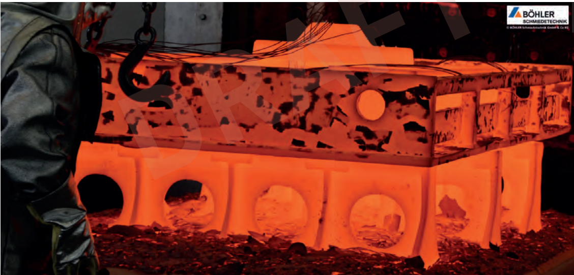
Fig. 2: Heat treatment measurements after forging with thermocouples in a turbine disk (© Böhler Schmiedetechnik)
